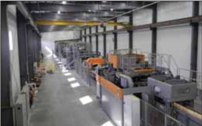
The new HewSaw® installed by Idaho Forest Group (IFG) allows for bigger logs with a 100-degree axis of motion, compared to only a 15-degree axis of motion on a traditional hewsaw, which makes it more like a CNC machine for wood.
