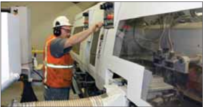
The state-of-the-art European equipment Interfor installed at Gilchrist included a Weinig H5000 high-speed moulder.
