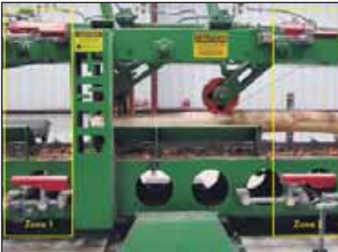
Once turned, log travels through two more scan zones and the scanned image is sent to the MillExpert canter optimizer to generate the best value solution.
