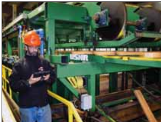
USNR's MyMill mobile machine control is being applied at Kalesnikoff Lumber to operate its new 70-bin sorter.
