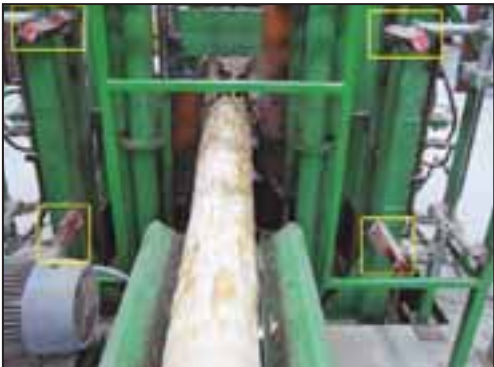
The log is scanned by 4 Smart TriCam sensors as it travels through the turners. The PGLR provides continuous feedback about the orientation of the log to correct rotation and achieve the target turn angle.
