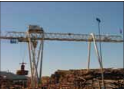
This log crane is capable of lifting an entire truckload from the truck and onto the yard.
