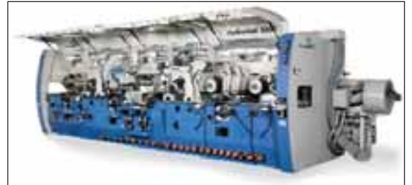
Interfor will be using its new Weinig H5000 moulder for all products except pattern. It can service up to 12 inches wide, providing edge control and finish quality that is unparalleled, according to Interfor.
