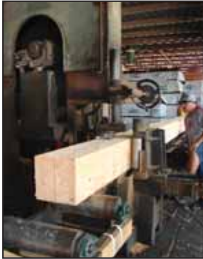
A 40-foot timber processes through Richardson's vertical band resaw.
