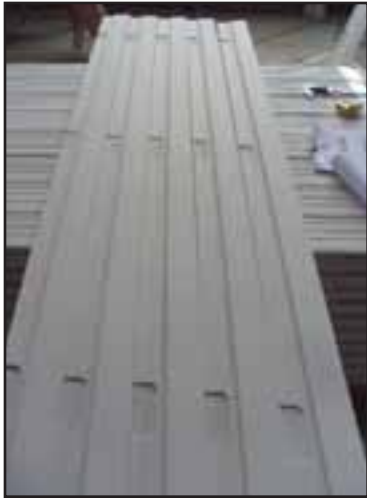
Weston Wood Solutions, Mississauga, Ont., stocks over 100 different jamb and window extension profiles, and can machine in-house head and sill dados to any specification. An image of mortised exterior jamb is shown here.
