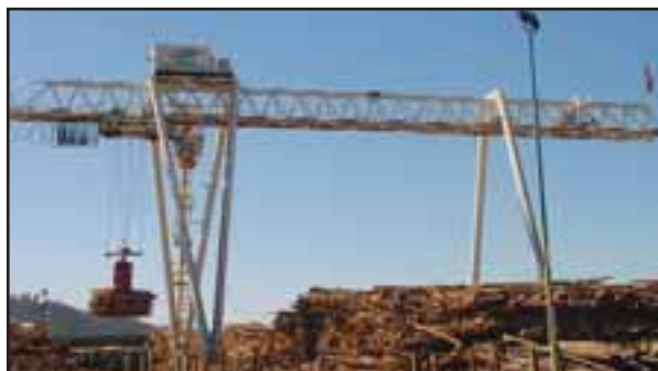
This log crane is capable of lifting an entire truckload from the truck and onto the yard.
