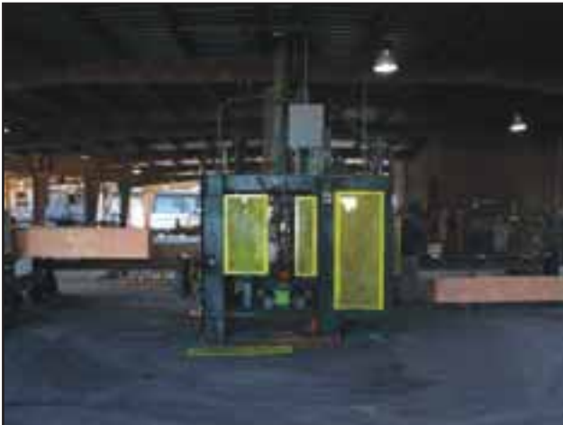
Custom built Tru-Ruf equipment provides a fresh cut appearance to the timber once it is processed.
