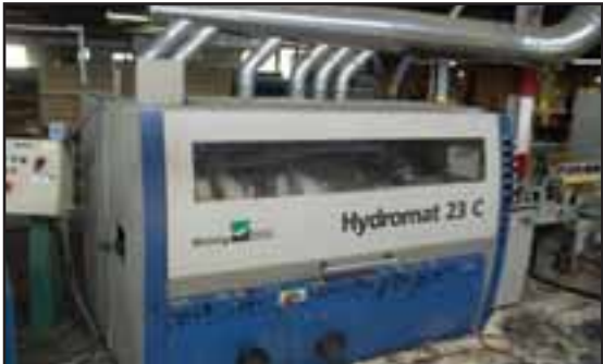
Mill Services recently installed a new Weinig moulder in its Cobleskill, N.Y., plant.
