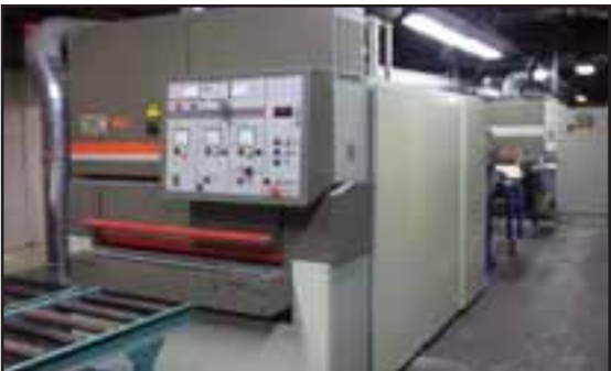
Mill Services offers a high quality finish on boards up to 48" wide using the company's new 52" DMC top and bottom sander.
