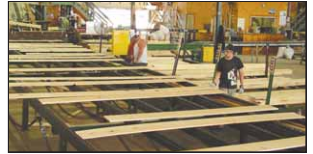
DiPrizio recently completed a 70-foot dry chain extension which will enable more sorts for their distribution customers across the U.S.
