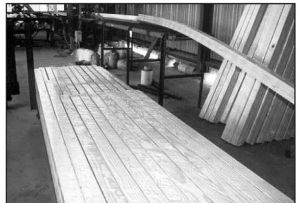
Center bead ceiling in C and Better grade is separated by lengths before it is sent through the shrink-wrap machine (background).
