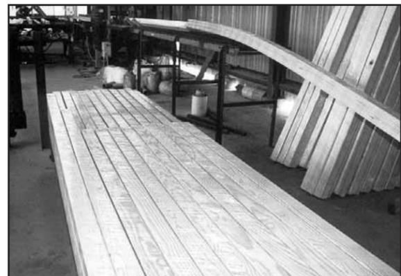
Center bead ceiling in C and Better grade is separated by lengths before it is sent through the shrink-wrap machine (background).
