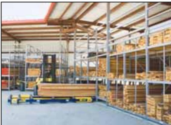
The Powerbin power deck at Big Creek Lumber loads a bundle of wood in less than a minute using only one worker.
