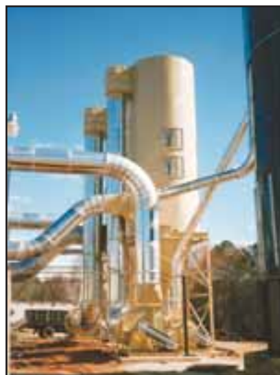
Southern Pneumatics, located in Knoxville, Tenn., recently installed this MAC baghouse at an architectural moulding plant in Roanoke, Ala.
