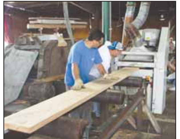
Richardson employees are shown surfacing all four sides (S4S) of a 2x12 Douglas Fir timber.
