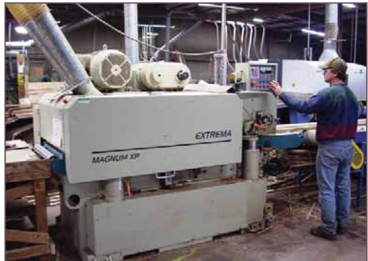
Operating the Extrema 225 Magnum XP surfacer, Manick programs board thickness.
