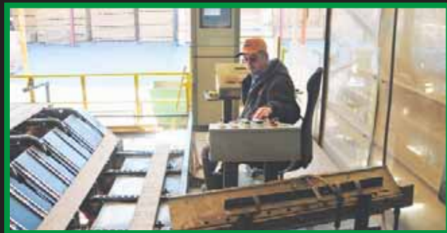
Ricky Parton operates Oaks Unlimited's computerized measurement and end tally kiln dried grading station.
