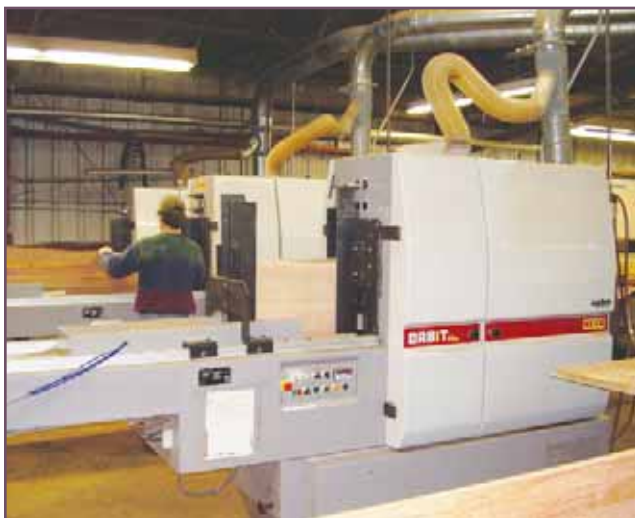
Production Superintendent Bill Manick loads blanks into an Ogden Orbit Plus frame saw.
