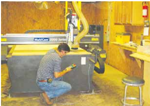
The MultiCam CNC machine enables Tom Julian's designs to be translated from CAD/CAM schematics into precision routing that allows for variable feed rates and operator-assisted adjustments when preparing materials for hand-crafted assembly on location.
