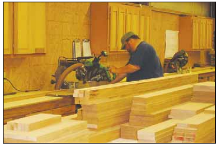
Precision cutting to length for an entire room full of custom millwork and cabinetry is one of the first stages in the Julian & Sons customized production process.
