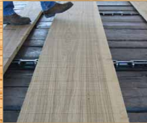
5/4 White Oak being graded on the green chain.
