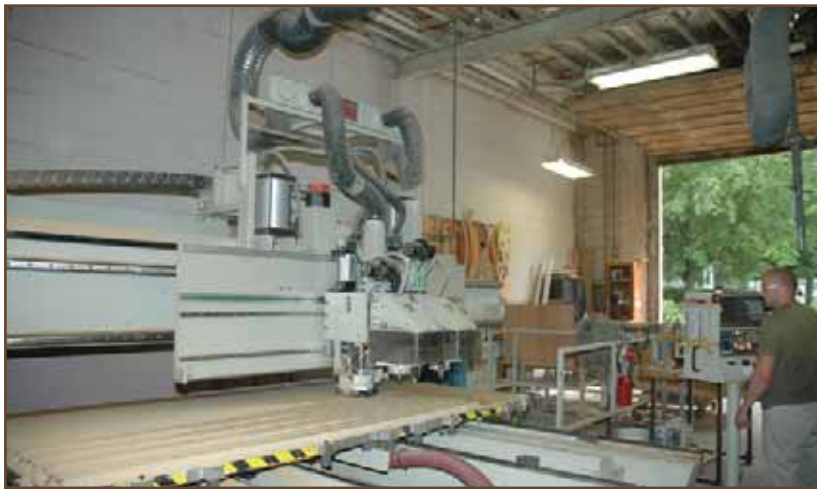
This is a view of the company's Komo computerized routing center with two 5x5 beds and two heads with eight tool changers on each.
