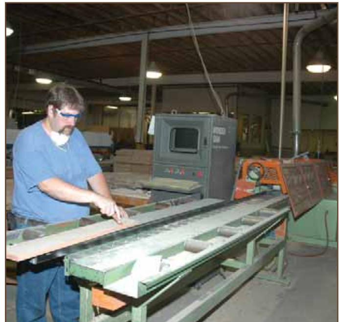
This is a view of an employee checking glue panel materials for defects before sending it into the Barr-Mullin computerized cutoff saw.
