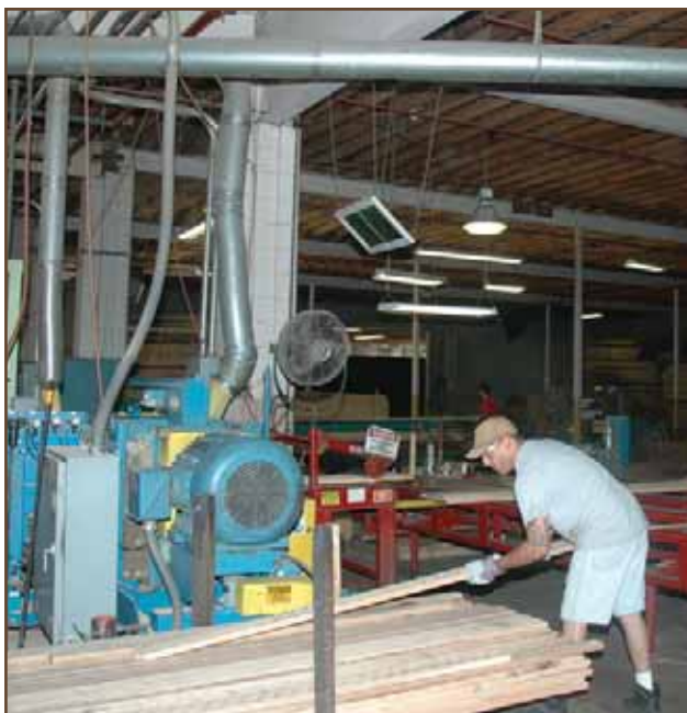
These are some employees ripping lumber on R.P. Wakefield's Barr-Mullin CompuRip computerized wood optimizer.
