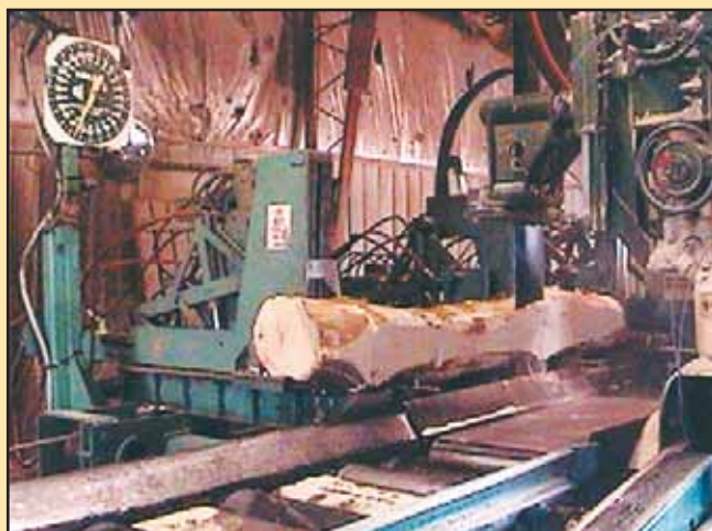
This is Bruggeman Lumber Inc.'s six-foot McDonough headrig cutting a large log into lumber.
