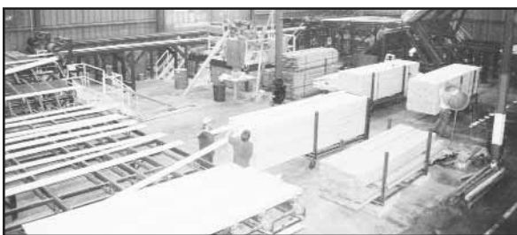
This is a view of Elk Creek Lumber Company's new planer line. The tilt hoist is shown in the top right hand side of the picture.
