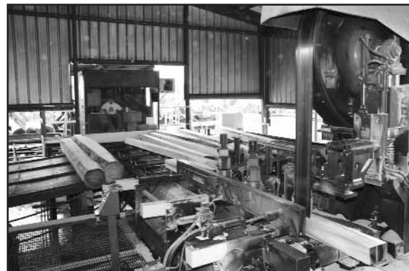
This is a view of our McDonough headrig that does a great job in manufacturing quality Hardwood lumber for our operation.
