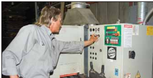
Owner Dwight Arithson prepares to run another batch of wood by adjusting the settings on the Weinig C-23 5 head moulder in the mill shop.
