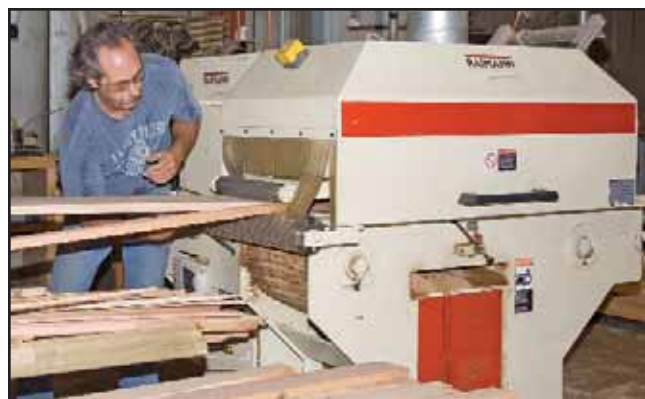
Mill Manager Jeff Wright guides a board out of the Raimann gang rip saw in the mill shop.
