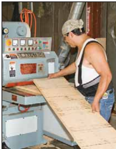
Employee Lupe Guzman feeds FAS Red Oak into the Northtech Double Helical Head Planer in the mill shop.
