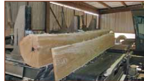
This is a view of Kepley-Frank Hardwood's circle saws cutting a large Appalachian log into lumber. The firm has three sawmills running at the company's headquarters.
